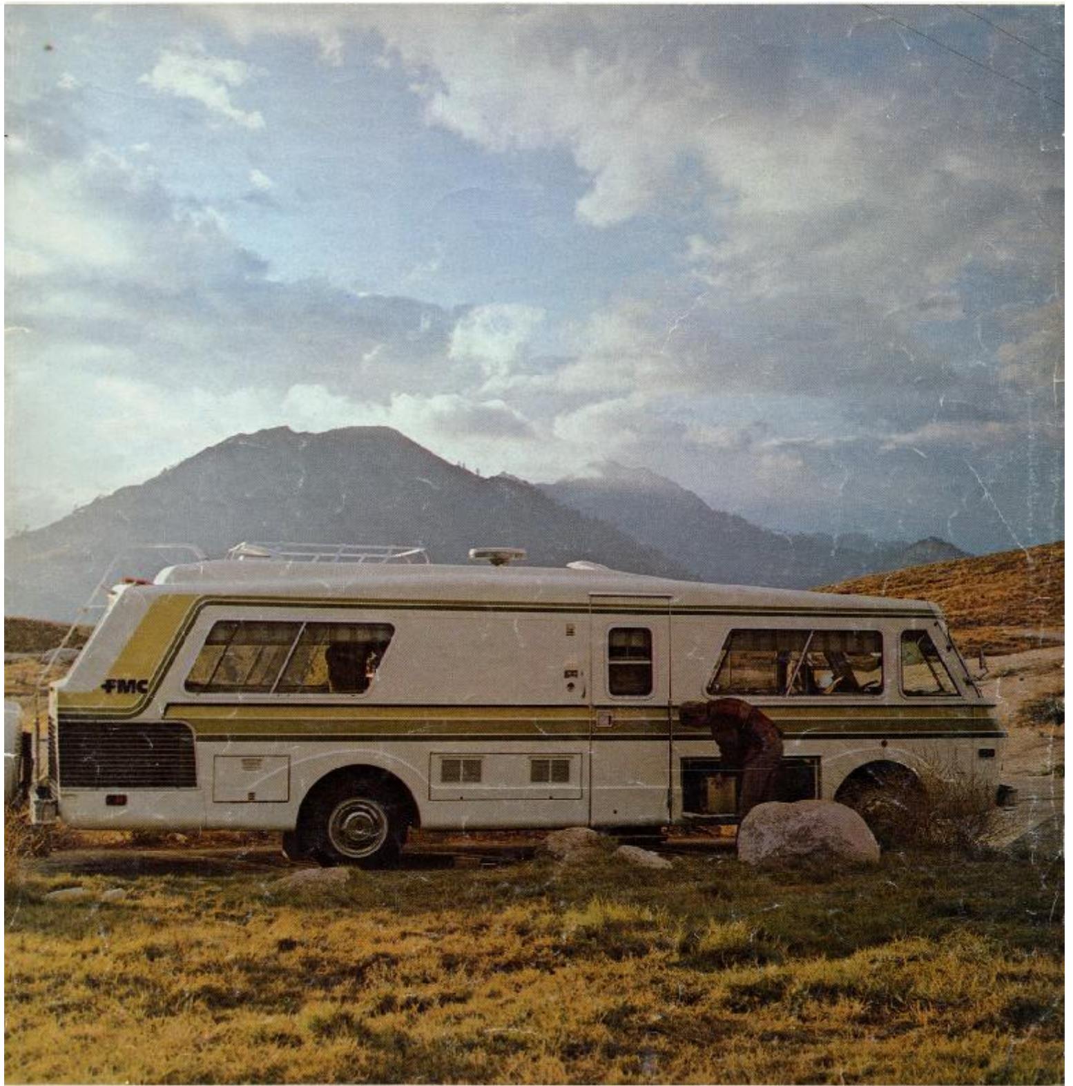
The FMC 2900R combines an attractive, aerodynamically styled coach and an unusual chassis with independent suspension.
