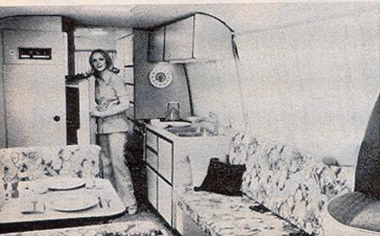
Dinette converts to double bed; couch back raises to make double berth. Main bedroom/lounge is at rear.
